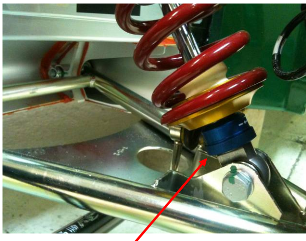
Rebound Adjustment – Clockwise Full Hard
